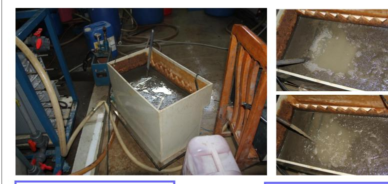
Before Fluid is Dark and contains huge chemical molecules which is difficult for later stage treatment
