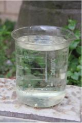
After 20 min. TMF-VD Filtration Process, the transparent clear water can be separated out. Which is high COD content and need to verify other Ion Content, performance for further use in mixing the New Coolant
